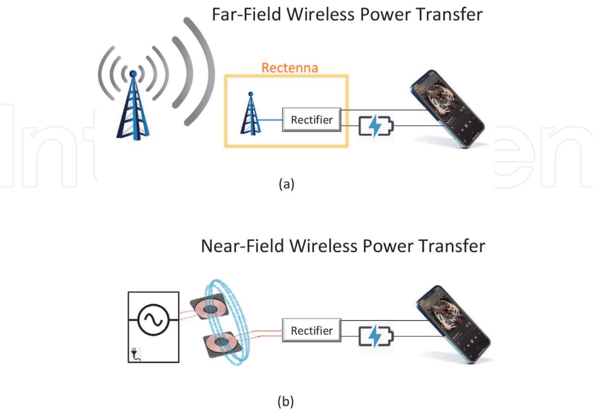
Figure 1. Representation of wireless power transmission in (a) far field where is highlighted the rectenna, and (b) near field.
