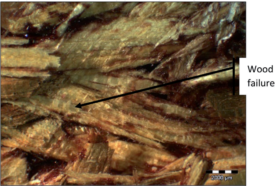
Figure 8. Failure occurred in the wood portion.
