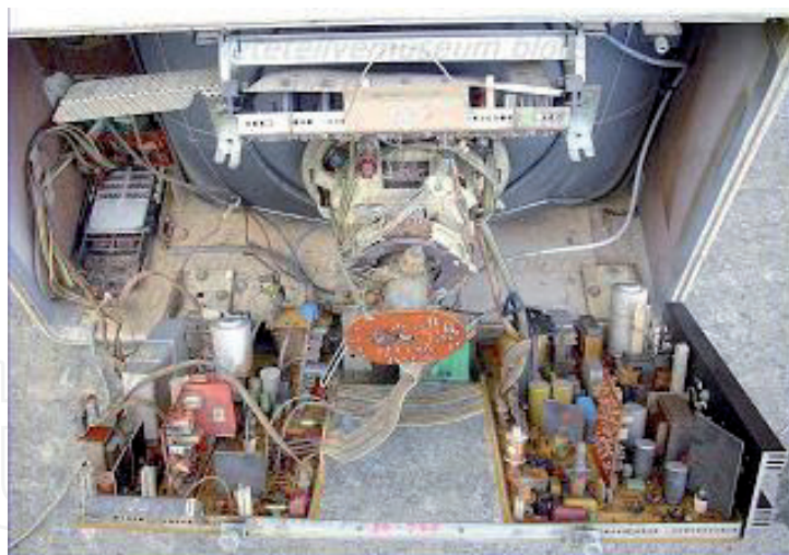
Figure 3. Digital TV receiver contains Mn-ferrites deflection yokes [15].
