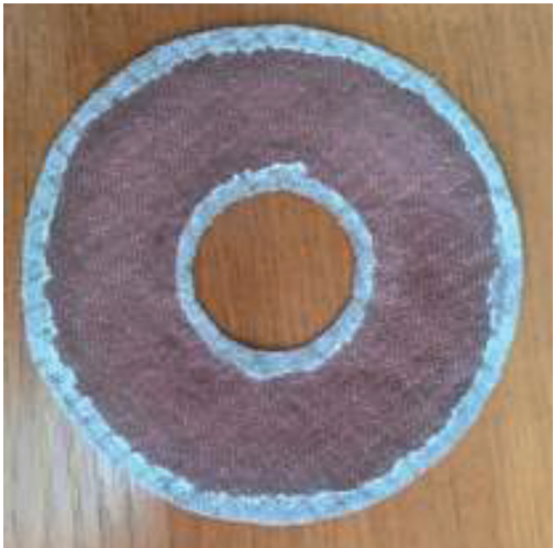
Figure 4. Same woven fabric with plasma copper coating.
