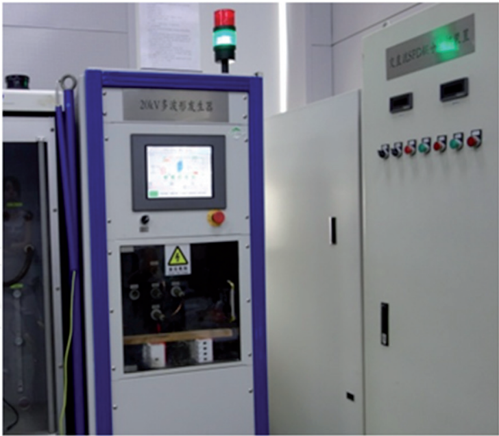
Figure 4. The multi-waveform lightning generator with the voltage of 20 kV.
