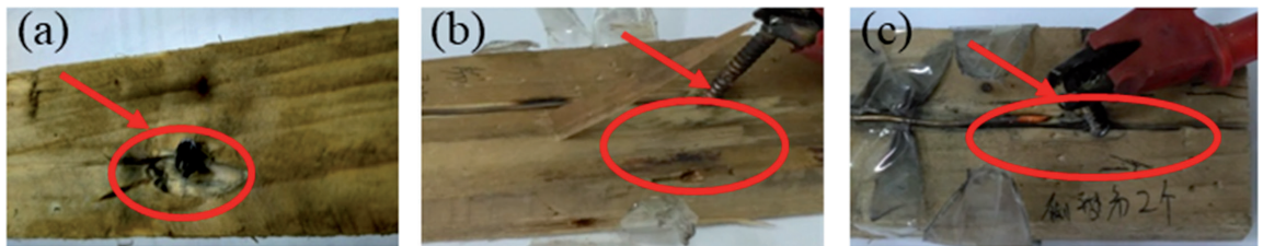
Figure 9. Impulse damage map of the timber with the water content of (a) 42.2%, (b) 47.6%, (c) 52.7%. (The red ovals represent the damage locations, and the red arrow faces toward Screw 2).
