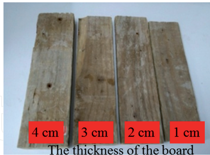
Figure 6. The timber board of ancient building with different thicknesses.
