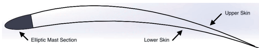
Figure 3. Twin-skin mainsail geometry.
