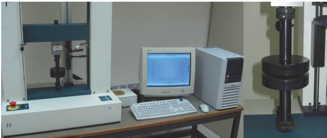
Figure 7. Setup for compression testing, using disc samples.
