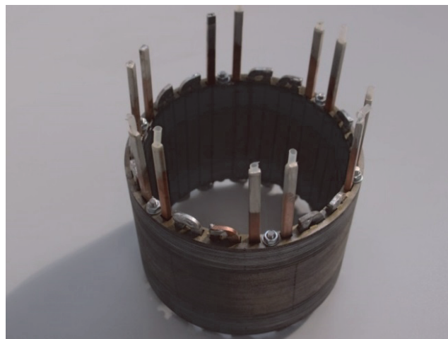
Figure 4. Solid bar winding, wave concentrated winding.
