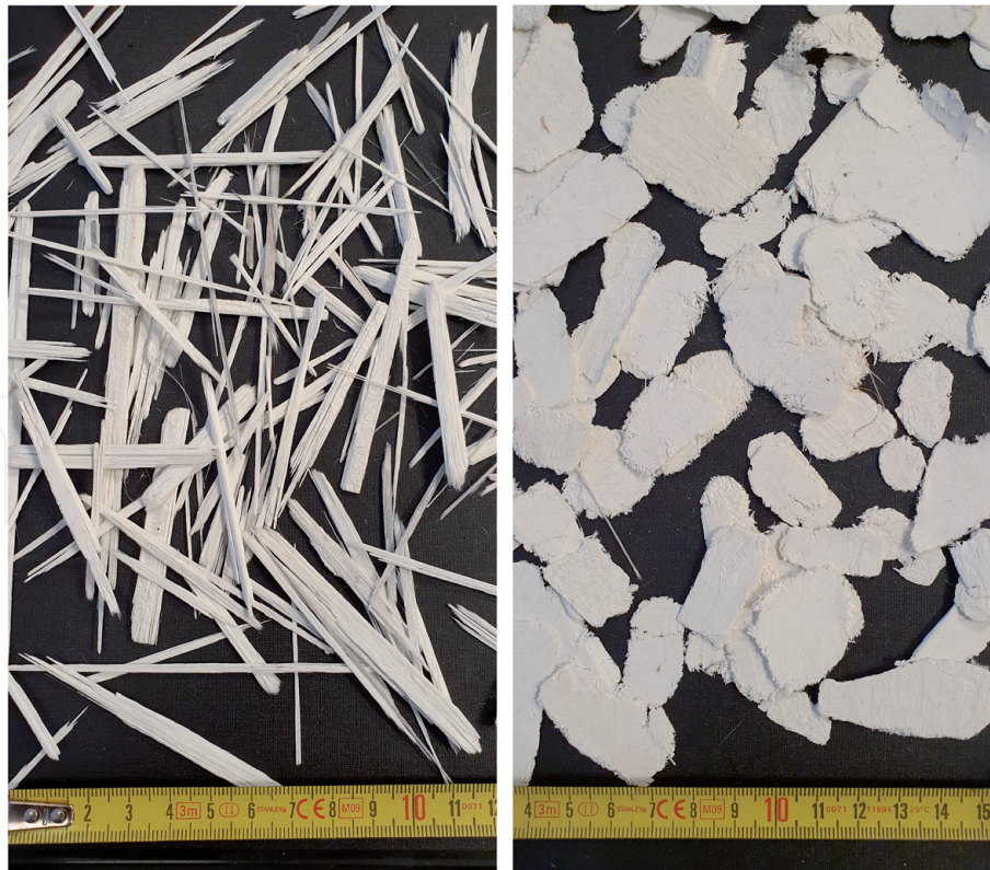
Figure 5. Shreds from rotor blades (left) and from boat hulls (right).
