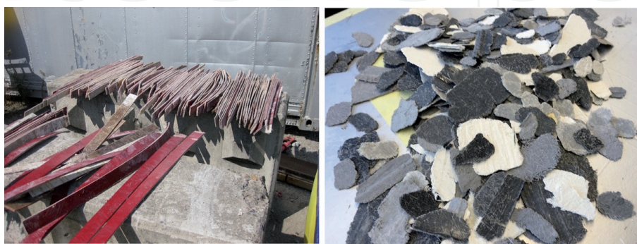
Figure 4. Panels sawn into strips or shredded into flakes [4].
