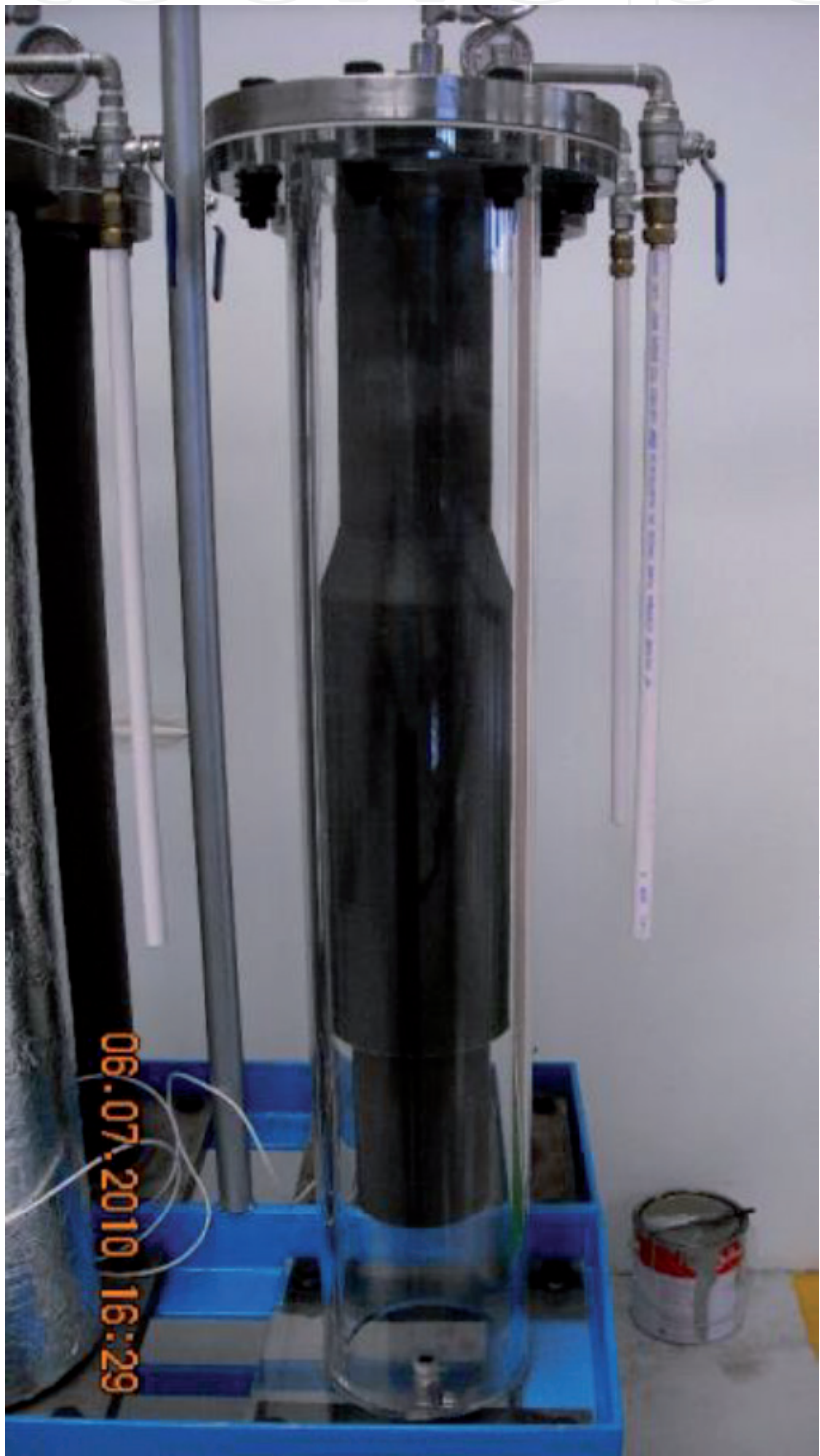
Figure 11. Perspex demonstration unit showing internal construction of other test units.
