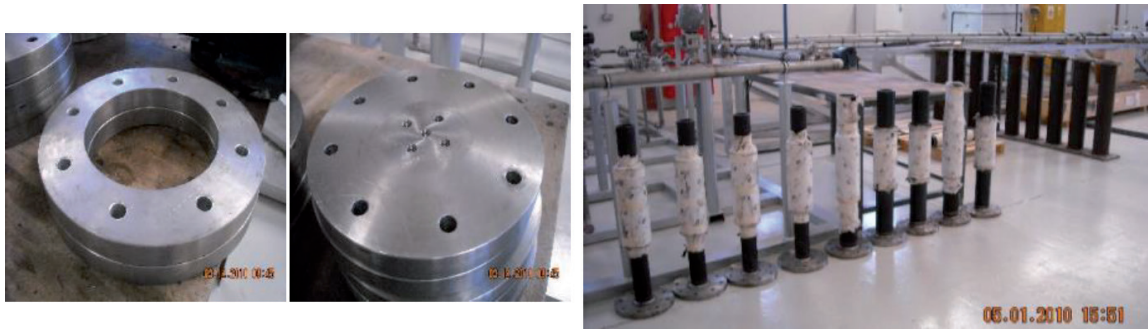
Figure 5. Fabrication of flanges (left); welding of flanges and bottom plates to packers and casings.
