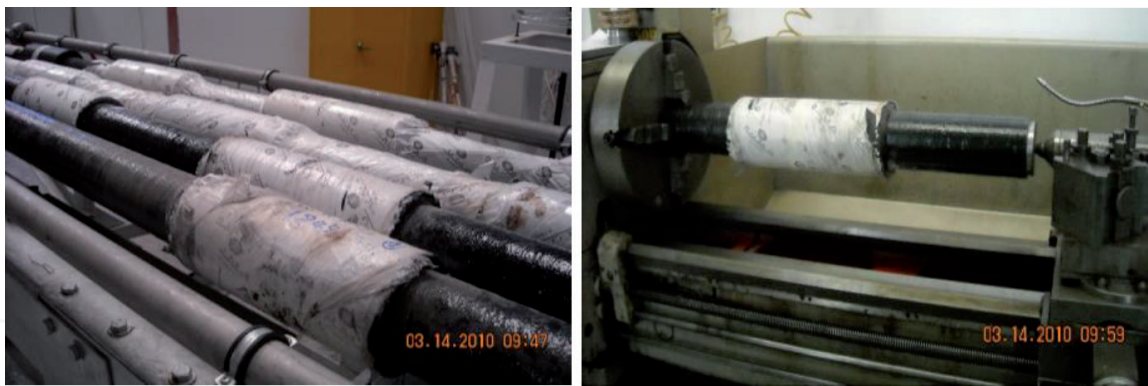
Figure 4. Full-length elastomer tubulars (left); sizing and beveling of elastomer packers (right).
