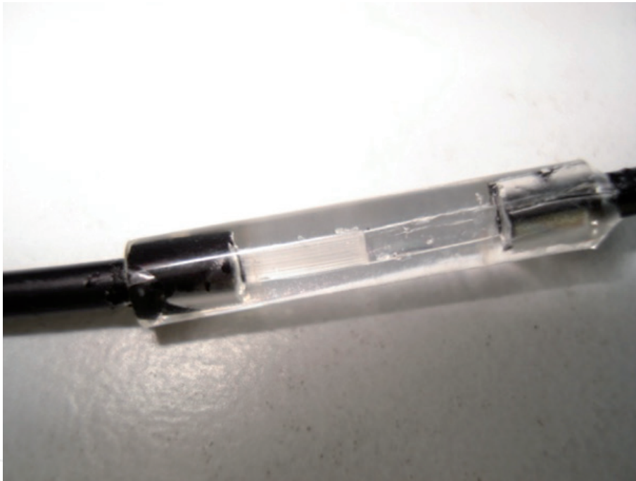
Figure 13. Optical splice with low attenuation.
