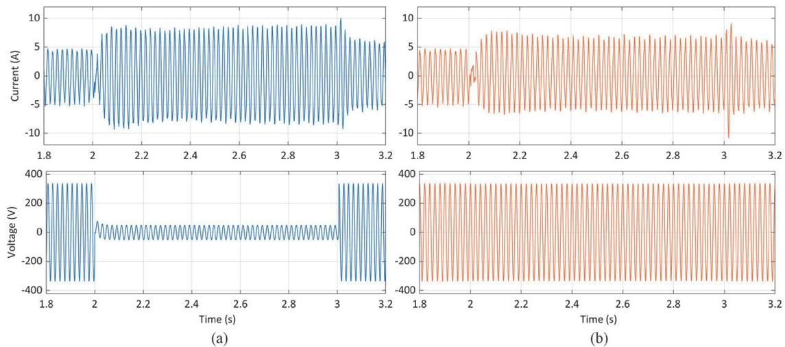
**Figure 6.** The solar inverter fault current for a line-to-ground fault (fault is from 2 to 3 sec). (a) Inverter current (A) – Top and terminal voltage (V) – Bottom of the faulty phase. (b) Inverter current (A) – Top and terminal voltage (V) – Bottom of the healthy phase.
