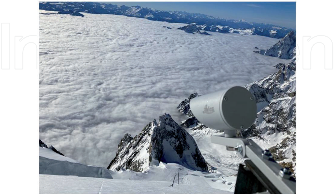
Figure 13. One of the prisms positioned on the Whymper Serac, pointing towards the robotic total station located in the hamlet of Planpincieux (photo: FMS).
