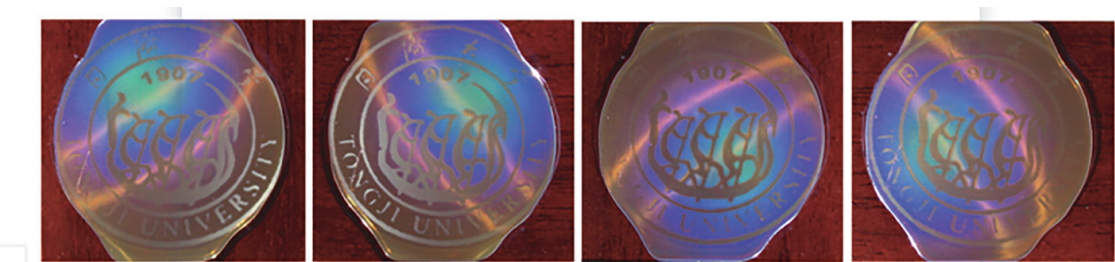
Figure 25. Digital photographs of the logo as the incident light is projected from different angles.
