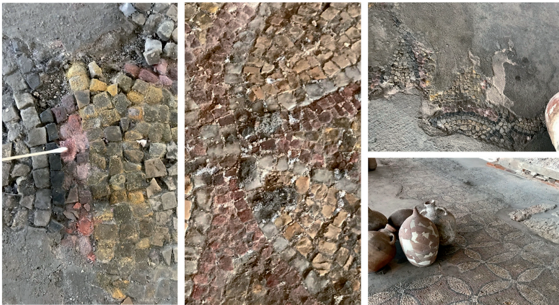
Figure 3. Appearance of the biological attack on tesserae.
