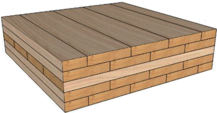
Figure 7. CLT panel layup with two parallel layers in outermost layers.
