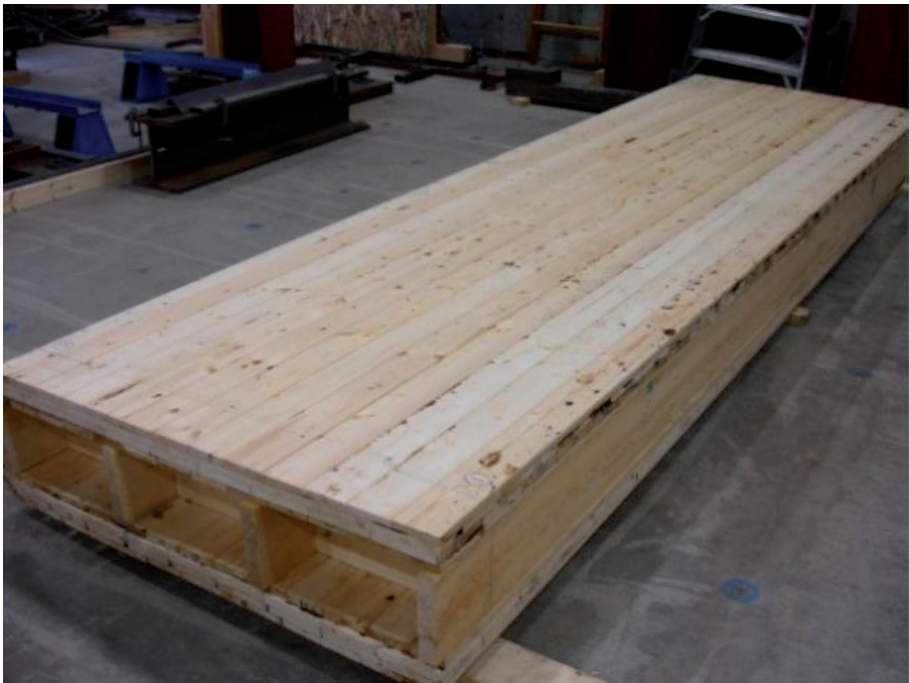
Figure 9. CLT panel layup with box-based configuration (adapted from Chen [11]).
