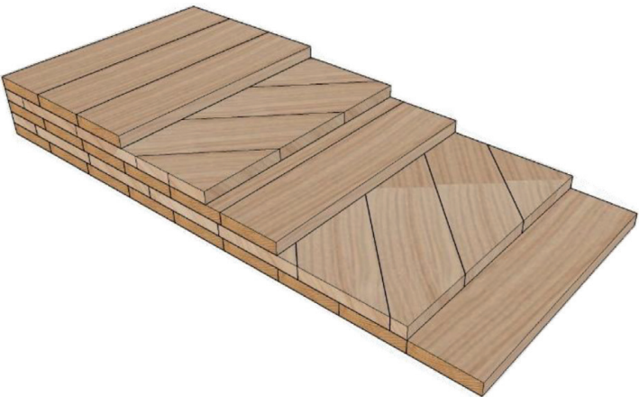
Figure 8. CLT panel layup with \pm 45^\circ alternating transverse layer configuration (adapted from Buck et al. [10]).
