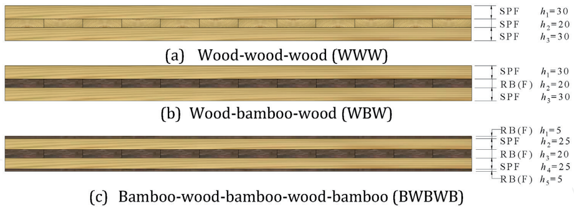
Figure 14. Configuration of bending specimen of CLT and CLTB (unit: mm). (a) Wood-wood-wood (WWW), (b) wood-bamboo-wood (WBW), (c) bamboo-wood-bamboo-wood-bamboo (BWBWB) (adapted from dong, [46]).
