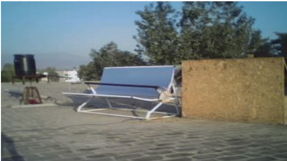
Figure 3. General view of parabolic trough solar water distillation unit.
