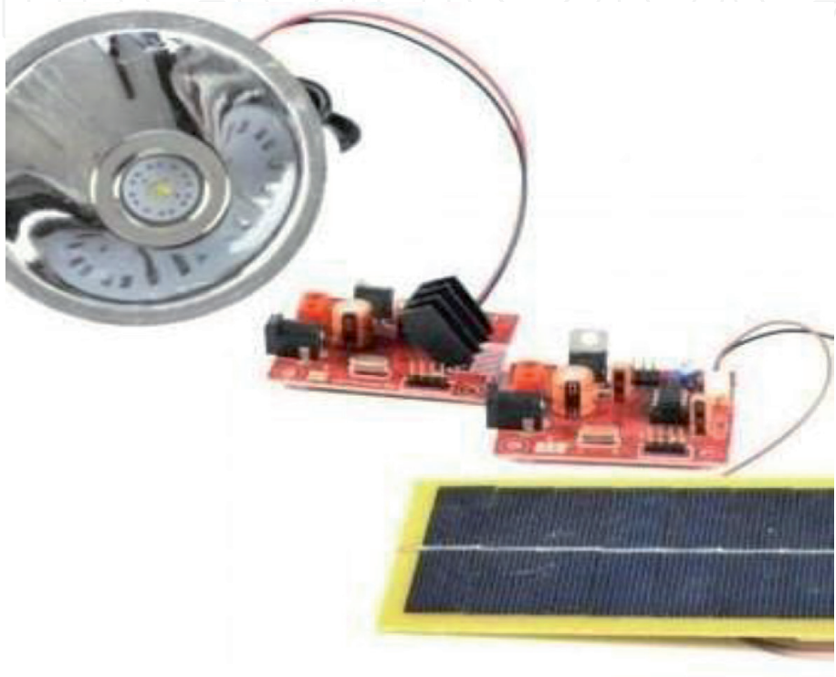
Figure 4. Working module of Li-Fi Tx and Rx via LED.
