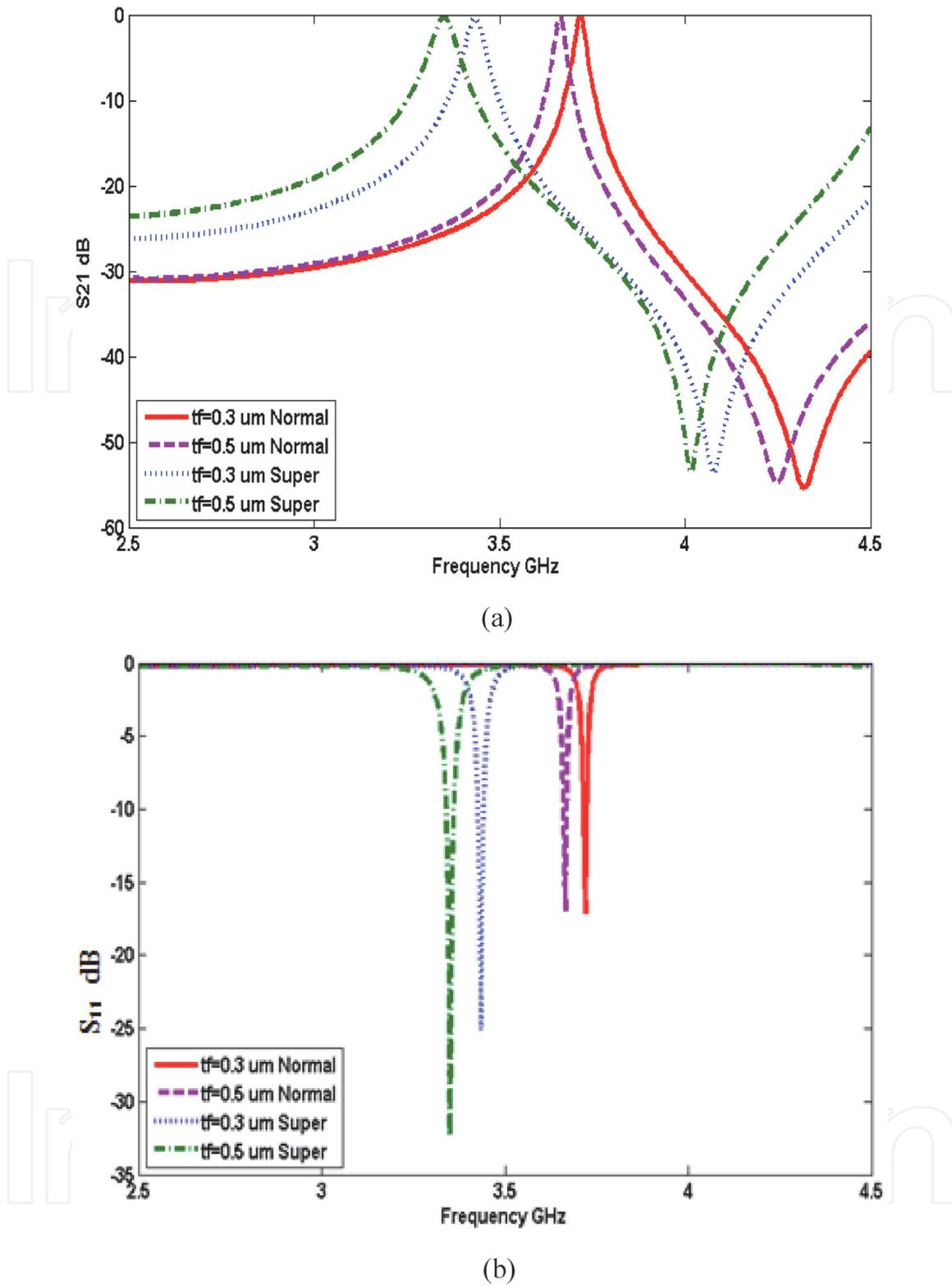
**Figure 10.** Variation of the magnitude of the transmission coefficient with the frequency at a different ferroelectric thickness  $t_{ferro}$ . (a)  $S_{21}$ . (b)  $S_{11}$ .
