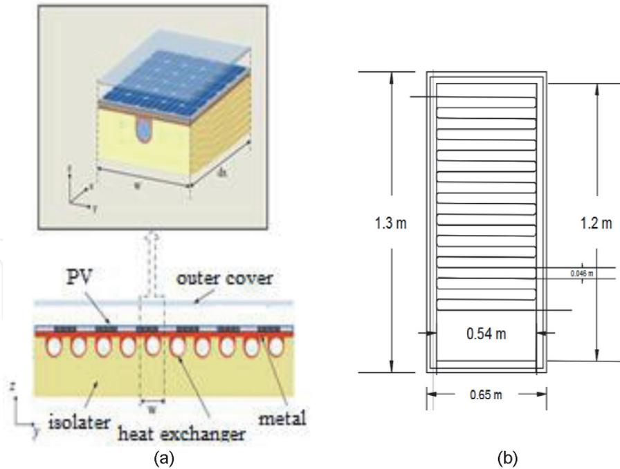
**Figure 6.** A diagram of the parts of the solar collector (PV/T collector). (a) Side clip of solar cell and heat exchange. (b) Dimensions of heat exchanger.
