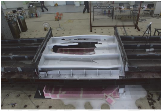
Figure 22. Deformed shapes of the tested structure at the ultimate limit state obtained from the test and the FE analysis with brittle material model.
