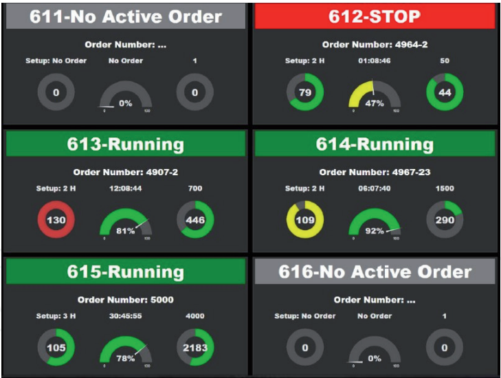
Figure 4. An example of the original production digitalization system prototype dashboard.
