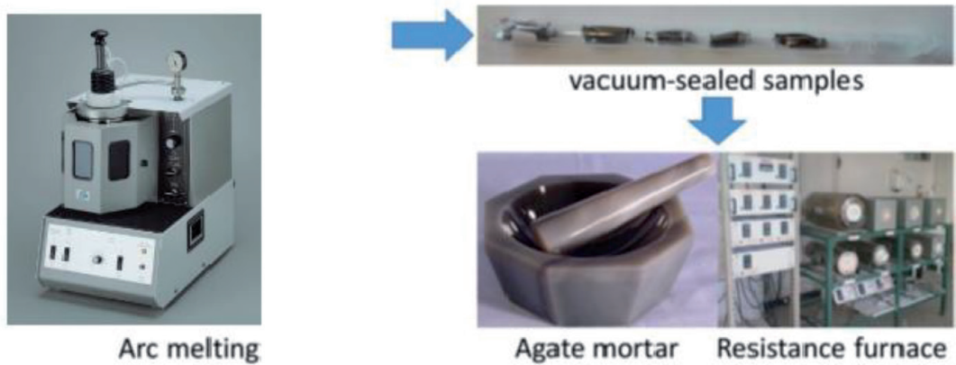
Figure 3. Synthesis steps using arc furnace method.
