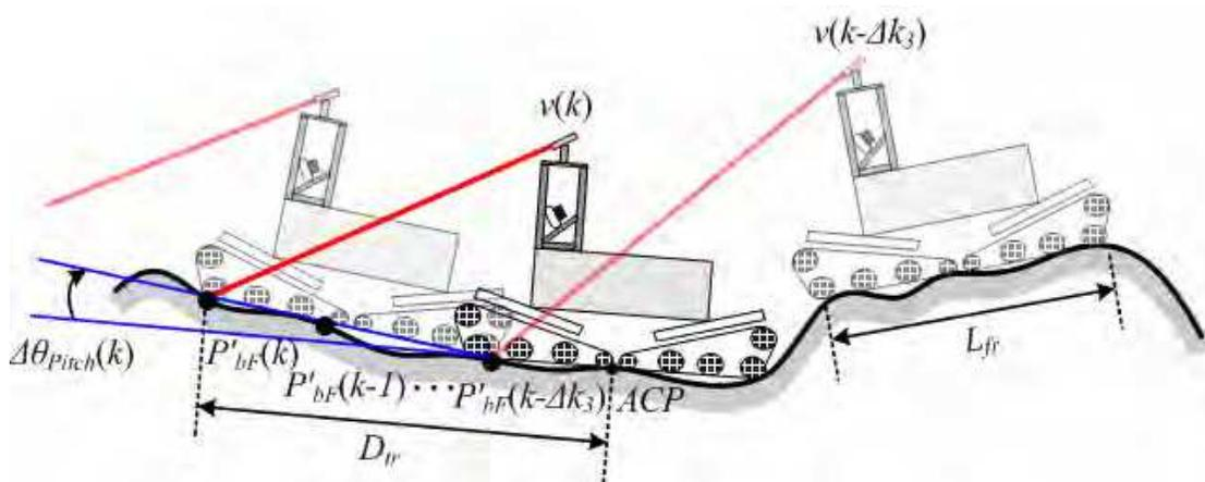
Fig. 11. Predicted pitch angle  $\Delta\theta_{Pitch}(k)$  at a distance of  $D_{tr}$  relative to the pitch angle at time  $k$  by using interpolated points  $P'_{bF}(k)$  and  $P'_{bF}(k-\Delta k_3)$  at times  $k$  and  $k-\Delta k_3$ , respectively.
