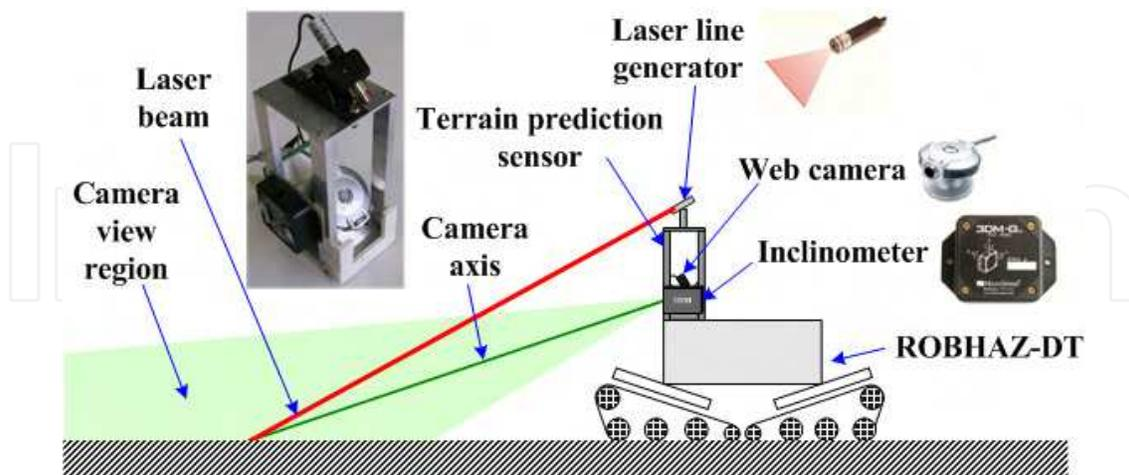
Fig. 4. Low-cost terrain prediction sensor module attached to the ROBHAZ-DT.
