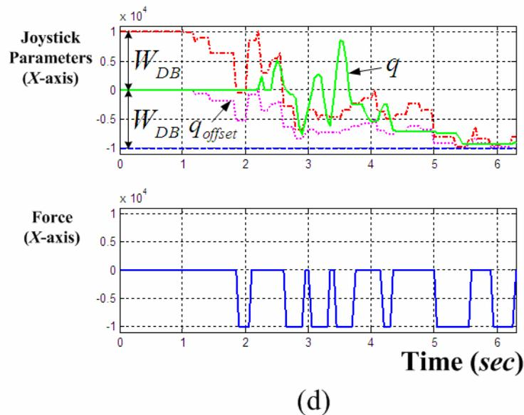
Fig. 23. Experimental results about turnover prevention ( $W_b=48$  cm and  $h_2=70$  cm): (a) Terrain parameters at a distance of  $D_{tr}$  in front of the agent, (b) rotational and translational velocities, (c) joystick parameters about the Y-axis, and (d) joystick parameters about the X-axis.
