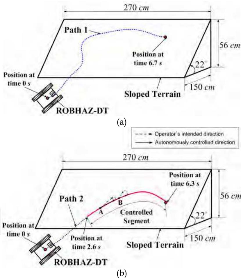
Fig. 21. Resultant paths of the ROBHAZ-DT moving on the sloped terrain: (a) Path1 for  $h_1=25$  cm, and (b) Path2 for  $h_2=70$  cm where the solid line segment indicates the controlled path for turnover prevention.
