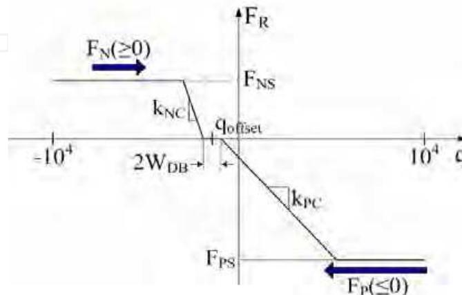
Fig. 19. Parameters of the position-based force  $F_R$  for the joystick position  $\mathbf{q}$ .
