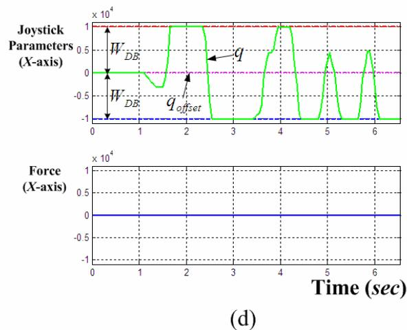
Fig. 22. Experimental results about turnover prevention ( $W_b=48$  cm and  $h_1=25$  cm): (a) Terrain parameters at a distance of  $D_{tr}$  in front of the agent, (b) rotational and translational velocities, (c) joystick parameters about the Y-axis, and (d) joystick parameters about the X-axis.
