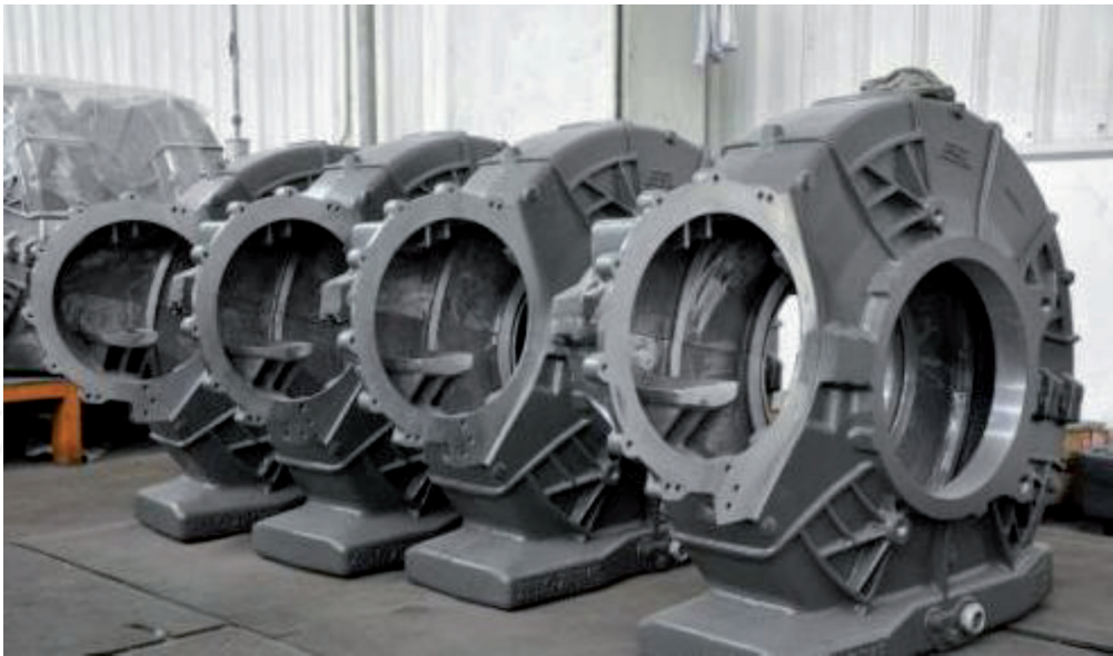
Figure 9. Typical aluminum gear boxes on CRH series high speed train.
