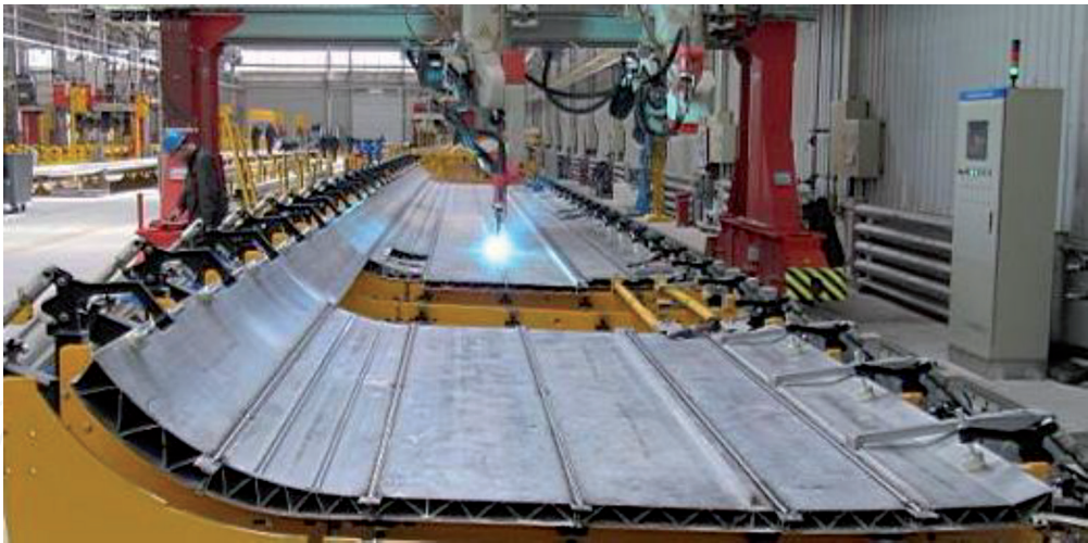
Figure 15. Automatically MIG welding process.
