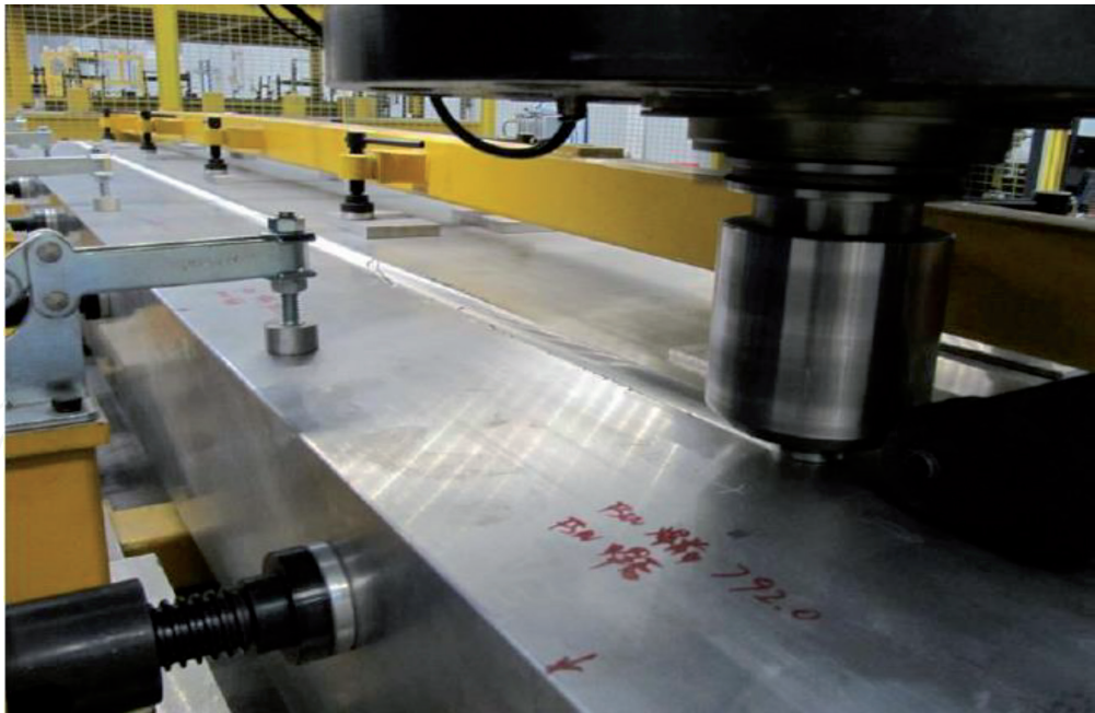
Figure 17. FSW process of a sleeper beam.
