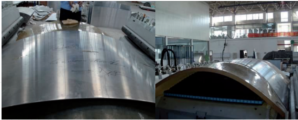
Figure 14. Skin drawing based on flexible multi-point die.
