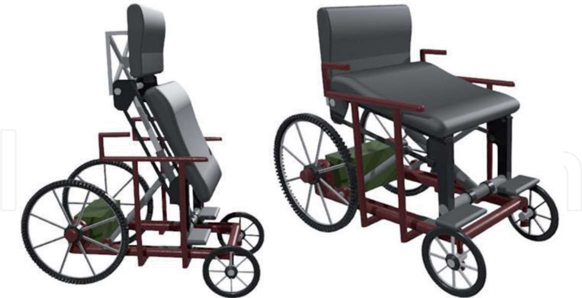
Figure 9. Linear actuator lift and recliner concept in seated and standing posture.
