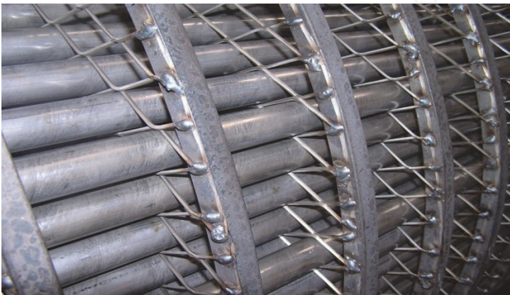
Figure 2. EMbaffle® design – One baffle fully supporting each individual tube.
