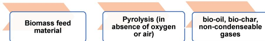
**Figure 10.** Flow diagram of pyrolysis methods [35].
