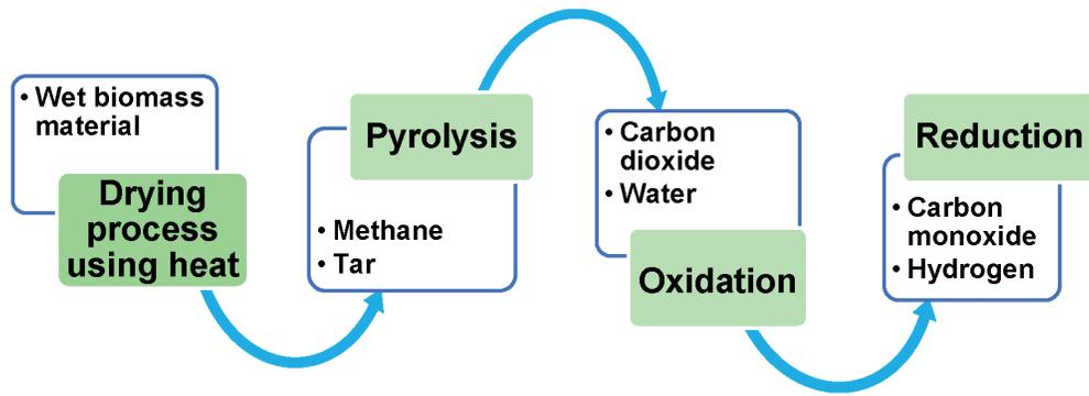
**Figure 8.** Energy generation process from biomass gasification method [33].
