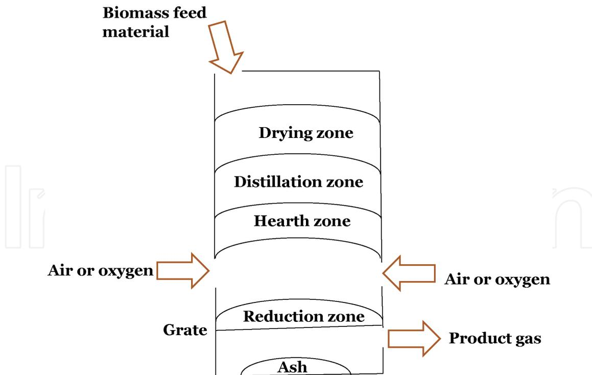
**Figure 15.** Gasification process using downdraft gasifier [54].
