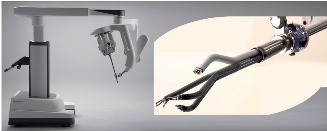
Figure 3. Single channel robotic arm with multiple instruments.
