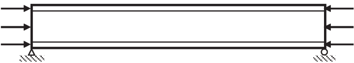
Figure 19. A biaxial edge load applied to faces and Core.
