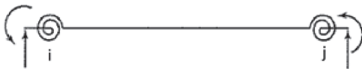
Figure 44. Frame element with semi-rigid connections.
