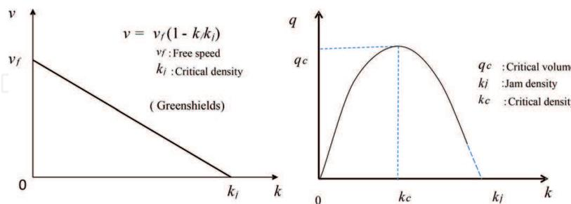
**Figure 5.** Fundamental traffic flow characteristics.
