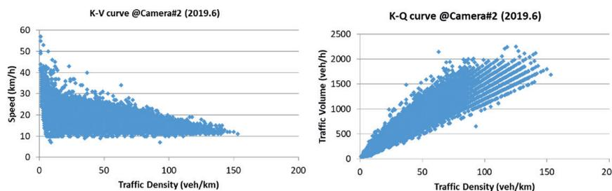
**Figure 6.** Fundamental traffic flow characteristics at camera#2.
