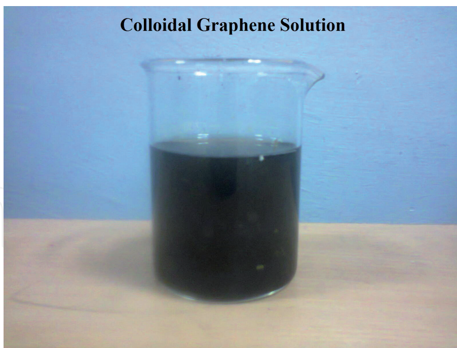
Figure 1. Colloidal solution of graphene in aqueous electrolyte.
