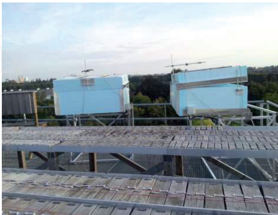
Figure 5. An arrangement of thermal boxes for surface radiation measurement.
