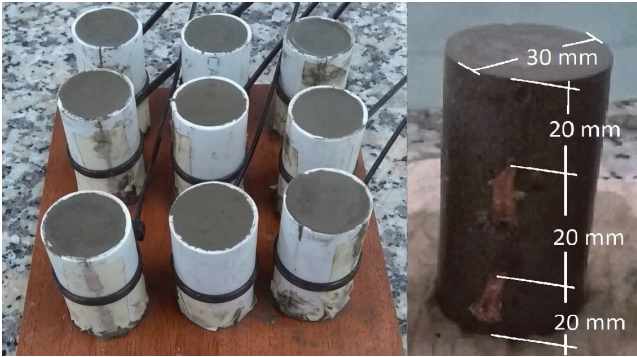
Figure 5. Molds and dimensions of cement cylinders.
