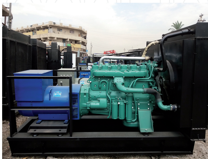
Figure 2. Locally assembled neighbourhood generator (Source: Author).
