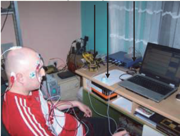
Figure 7. Experimental setup for BMI control of a robotic arm based on a CNV flip-flop.
