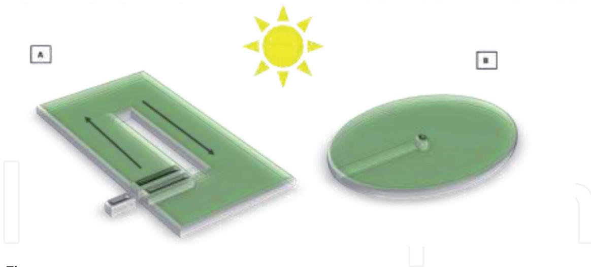
Figure 2. Open ponds photobioreactors. Raceway pond (A); circular pond (B). Source: authors.
