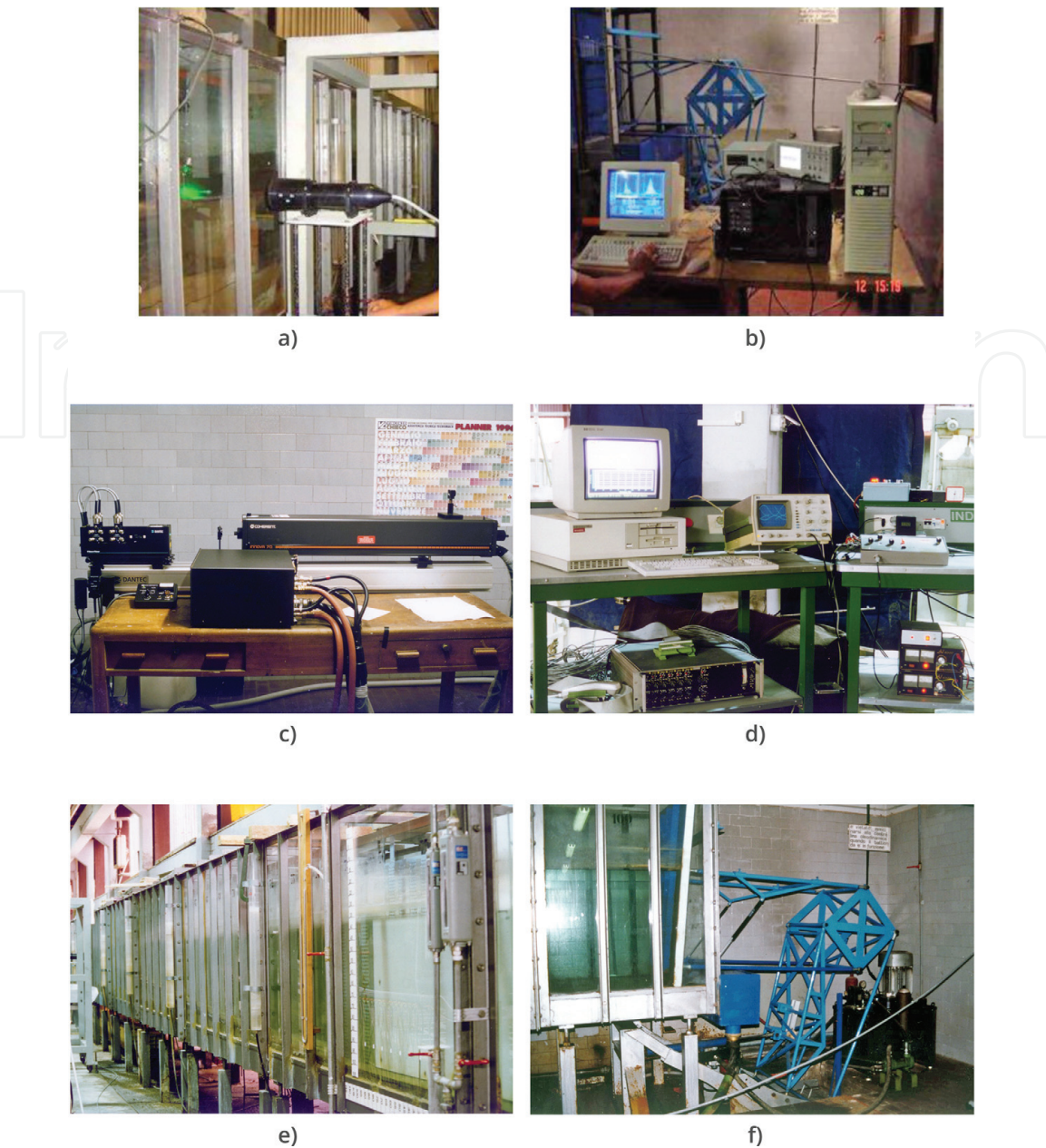
Figure 1. Experimental apparatus: (a) LDA probe; (b) DANTEC FVA signal processor and process computer; (c) laser coherent Innova and Dantec 2D fiber flow optics; (d) process computer with a AD/DA board for the wavemaker control; (e) a part of the wave channel; (f) the wavemaker.
