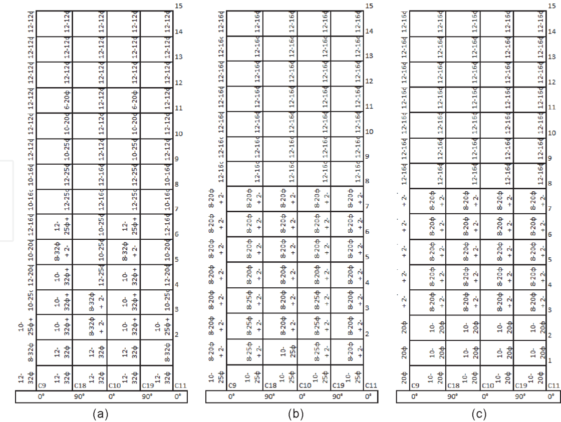
Figure 14. Comparison of reinforcement in columns. (a) IS code design. (b) ACI-318 code design. (c) EC8 design.
