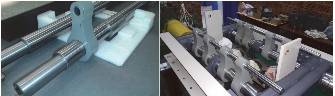
Figure 11. Connecting yokes mounted with the eccentric shafts.
