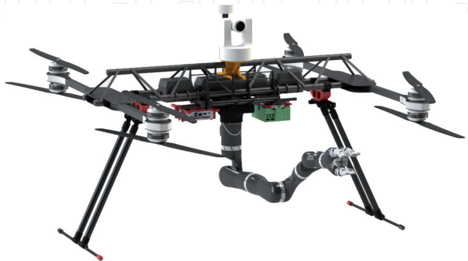
Figure 18. Aerial manipulation system with PTZ-camera.
