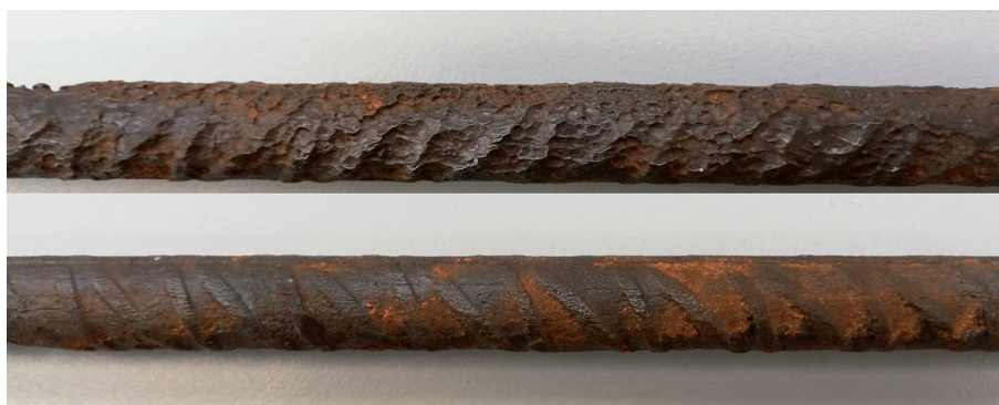
Figure 5. Corrosion damage on steel surface. Inner half of steel bar's circumference (up) - outer half of steel bar's circumference (down).
