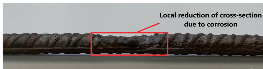
Figure 4. Local reduction of cross-section due to corrosion.
