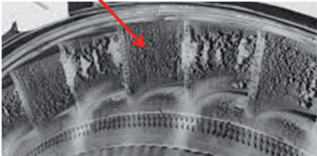
Figure 7. Erosion of compressor blades in gas turbine engine.
