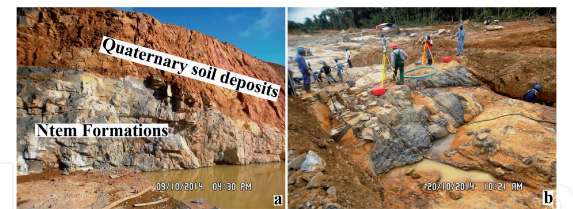
Figure 2. (a) Quaternary soil deposits underlain by Ntem formations that represent two geological units found in the whole dam site and (b) fractured and slightly weathered rock mass.
