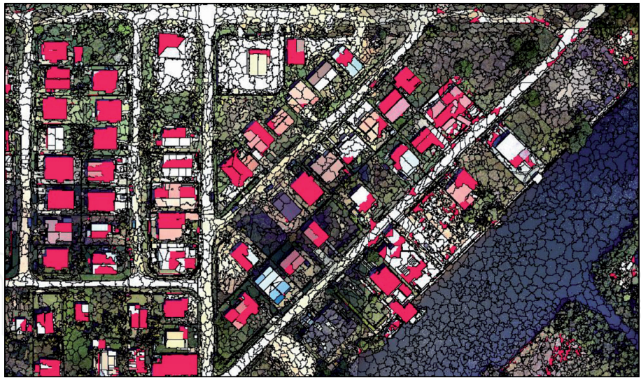
Figure 6. Building footprint extraction using PCA of RGB, NIR, slope and nDSM.
