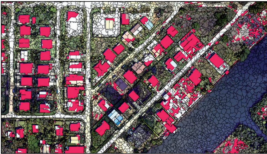
Figure 5. Building footprint extraction using PCA of RGB and nDSM.
