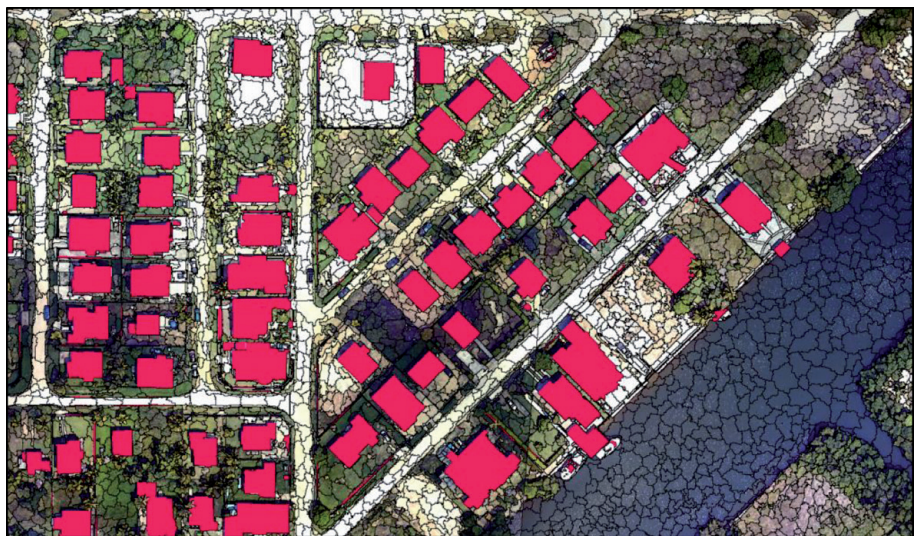
Figure 9. Building footprint extraction using PCA of RGB, NIR and nDSM.
