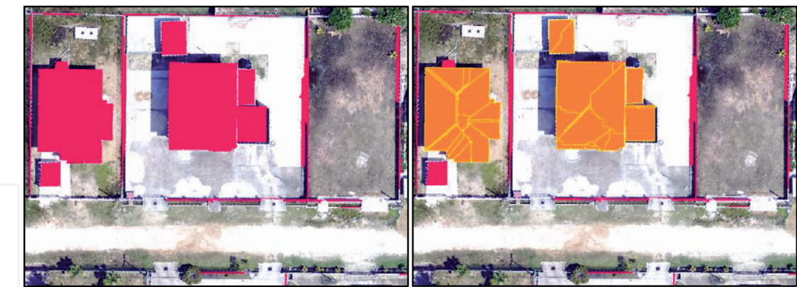
Figure 12. Rule-based extraction of building footprints.
