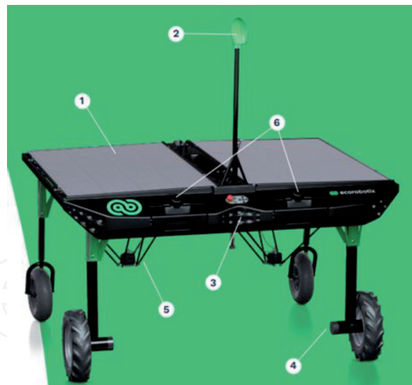
Figure 21. Ecorobotix components. (1) Photovoltaic panels, (2) camera and artificial vision for steering and detection, (3) navigation by GPS and sensors, (4) electrical drive system, (5) rapid robotic arms with sprayers, and (6) tanks for two different products. Source: Ecorobotix [45].
