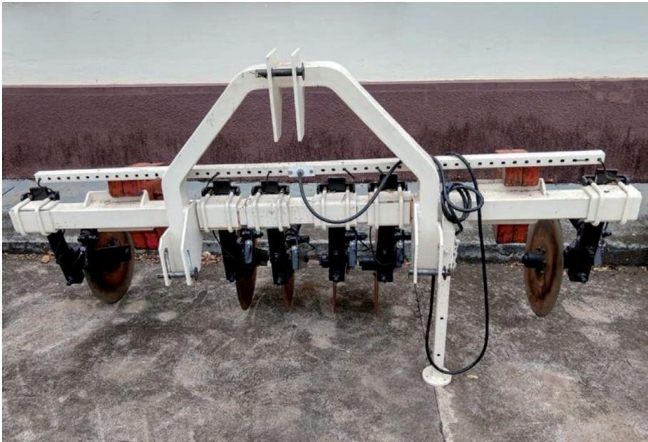
Figure 5. Veris Platform® 3100 to measure the electrical conductivity of the soil. ESALQ/USP, Piracicaba, SP, Brazil.
