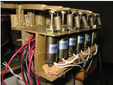
Fig. 11. Solenoid (with holding power of 1.5 pounds) attached to Jasche.
