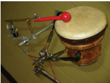
Fig. 15. Sample Motion Module Architecture: drumstick controlled by solenoid
