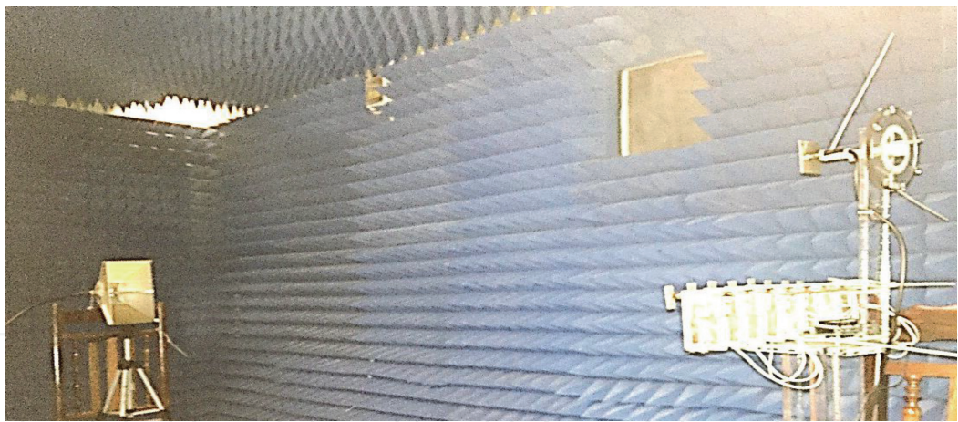
Figure 31. Array antenna measurement in anechoic chamber.
