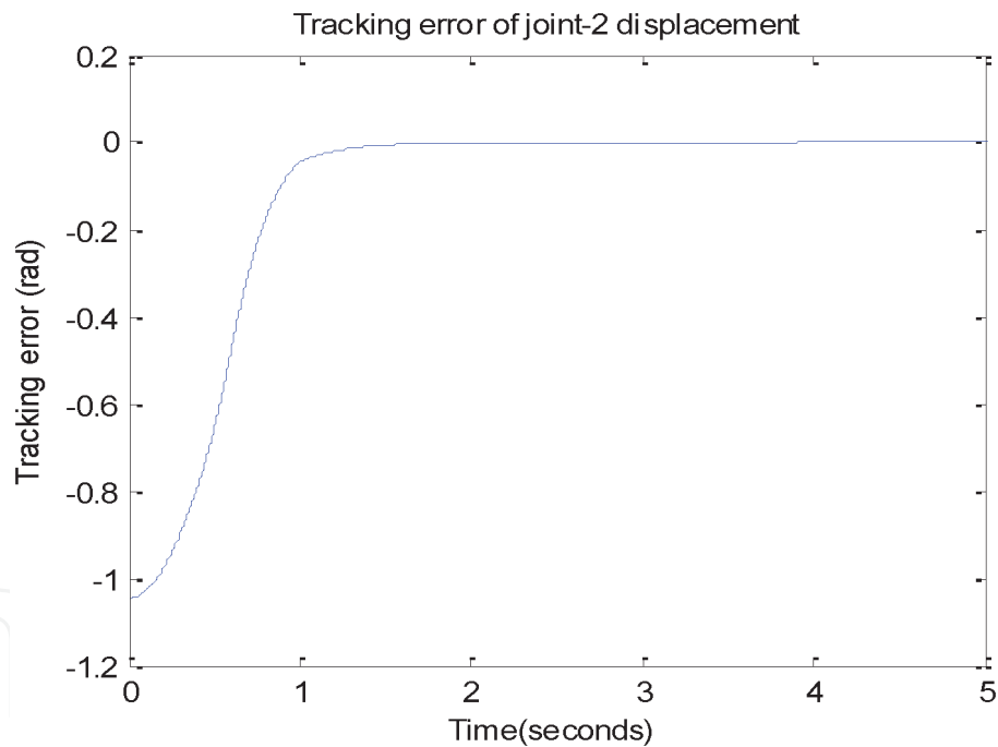
Figure 25. Tracking error of Joint 2 displacement under SMC of the robot manipulator.
