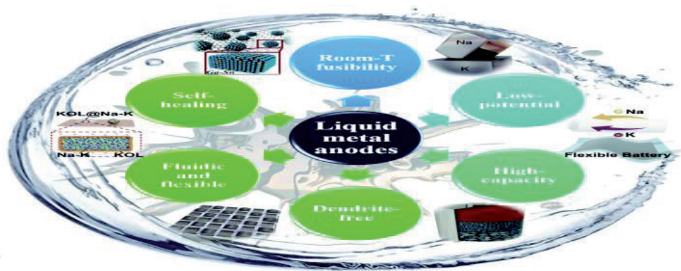
Figure 2. Room-temperature liquid metal alloy matrix for flexible battery/energy store.
